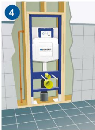
4 Install the tank and carrier.
