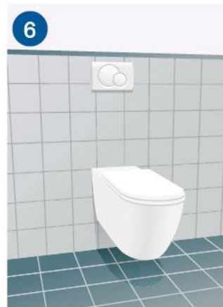
6 Mount the flush plate and wall-hung toilet.
