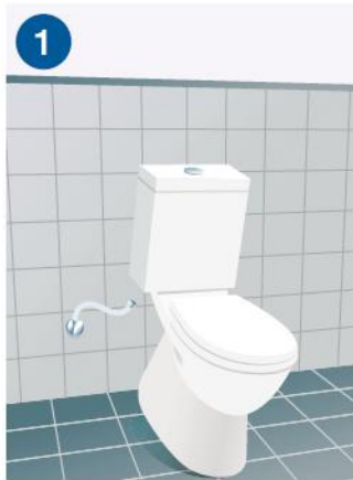
1 Remove the old toilet and tank.
