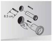
Ensure that the rag-bolts are projecting to a distance of at least 8.5 cm from the walls. Fix the connectors to the respective holes.
