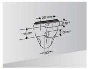
Fix the rag-bolts in the wall at the distances as per the dimensions of the products. Follow the same procedures for drilling the inlet and outlet holes.
