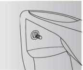
After tightening, ensure that there is no gap between the appliance and the wall. If so, use sealant to fill the
