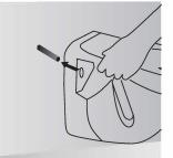
Ensure that the rag-bolts are projecting to a distance of at least 8.5 cm from the walls. Fix the connectors to the respective holes.
