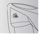
After tightening, ensure that there is no gap between the appliance and the wall. If so, use sealant to fill the gap. Tighten the washers and nuts using spanner.
