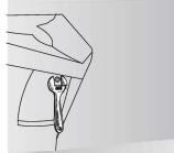
Fix the closet in the rag-bolts and insert the washers and nuts.
